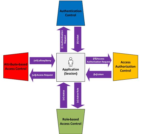
Fig. 1. Proposed Access Control Model
