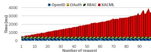
Fig. 5. Effects of increasing simultaneous requests in the proposal entities.
