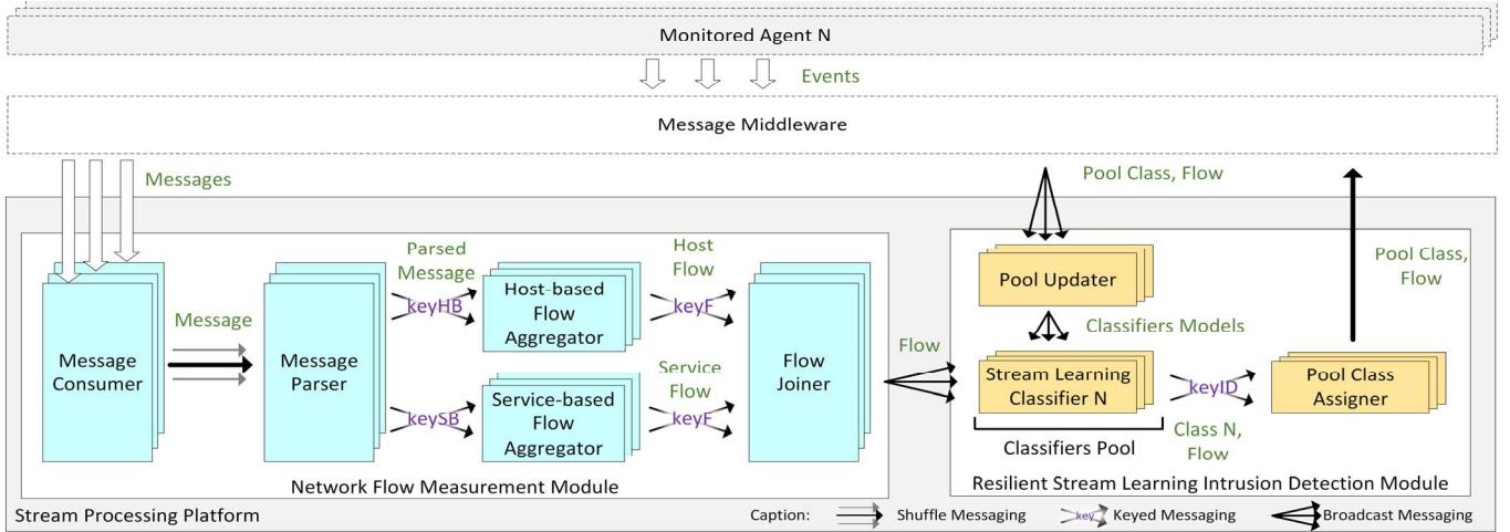
Figure 1 – Overview of the proposed real-time network traffic measurement architecture.
