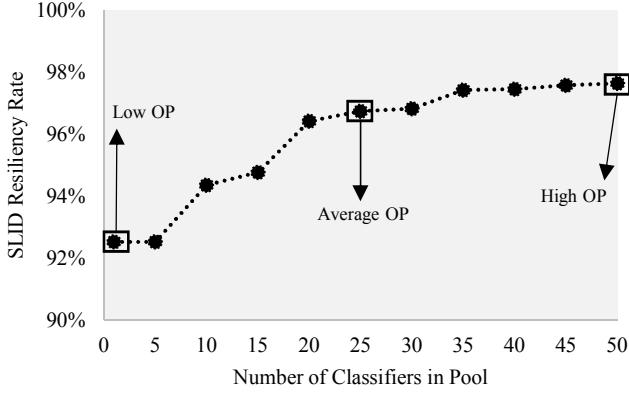
Figure 2 – Tradeoff between SLID resilience rate and classifiers in pool.
