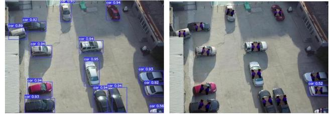
(a) UAV object detection without adversarial patches (b) UAV object detection with adversarial patches
